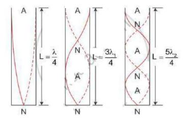
In the first mode of vibration of the air column, there is one node and one antinode as shown in the figure above.
