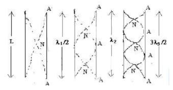
The simplest mode of vibration is the fundamental mode of vibration. (in above fig a ) In this case one node & two antinodes are formed. If  $\lambda_1$  be the corresponding wavelength &
