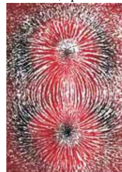
Figure 5.2 Systematic Arrangement of Iron Filings Representing Magnetic Field Lines of a Bar Magnet
