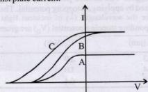
A and B will have different intensities while B and C will have different frequencies
