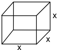
$$\begin{aligned}\text{T.S.A} &= 2(x^2 + x^2 + x^2) = 6x^2 \\ \text{C.S.A} &= 4x^2 \\ \text{Volume} &= x^3 \\ \text{Length of diagonal} &= x\sqrt{3}\end{aligned}$$
