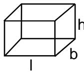
$$\begin{aligned}\text{T.S.A} &= 2(lb + bh + hl) \\ \text{C.S.A} &= 2h(l + b) \\ \text{Volume} &= l \times b \times h\end{aligned}$$
