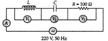
As V  $_{\rm L}$  = V  $_{\rm C}$  = 300V ,therefore the given series LCR circuit is in resonance.  $\therefore V_{R} = V = 220V$  $Z = R = 100\Omega$ Current, I =  $\frac{V}{Z} = \frac{220V}{100}\Omega = 2.2A$ Hence, the reading of the voltmeter V  $_3$  is 220 V and the reading of ammeter A is 2.2 A
