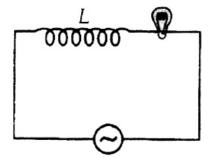
As the iron rod is inserted, the magnetic field inside the coil magnetizes the iron increasing the magnetic field inside it. Hence, the inductance of the coil increases. Consequently, the inductive reactance of the coil increases. As a result, a larger fraction of the applied AC voltage appears across the inductor, leaving less voltage across the bulb. Therefore, the brightness of the light bulb decreases.
