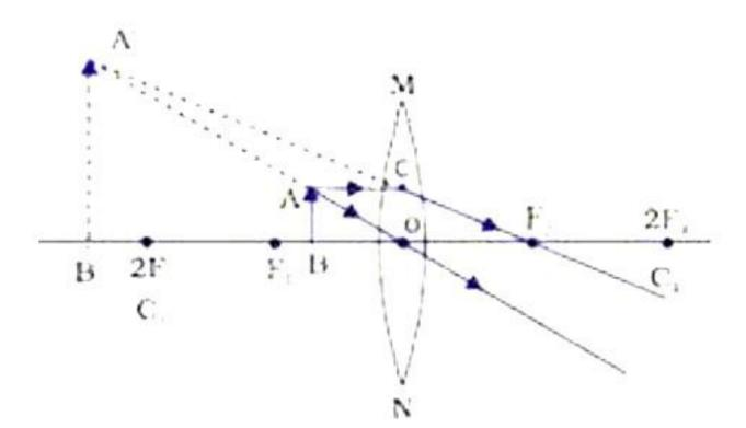
Nature and size of the image: Virtual and erect and Enlarged Position of the image: Beyond Fon side as the object.
