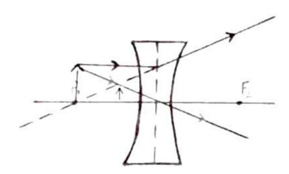
At the end, the image will be smaller, virtual and erect.
