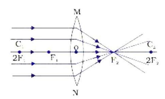
Nature and size of the image: Real and inverted and highly diminished Position of the image: Formed at focus F.
