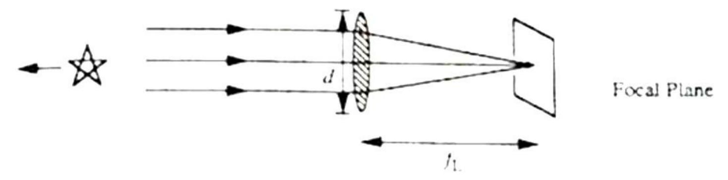
Since the light rays are incident from a distant object and nearly parallel, the image of it formed on the wall is read directly by the meter scale. This gives the approximate focal length of the scale.
