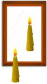
Candle image in mirror is erect, of same size and at same distance
