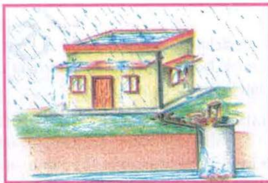
Fig-1 (D) : (B) Recharge through abandoned dug well (Rooftop rainwater harvesting)
