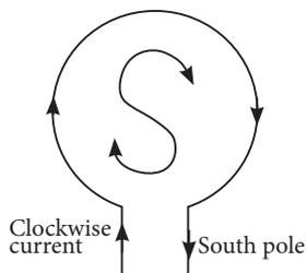
(c) By Fleming's left-hand rule, the direction of the magnetic field at the centre of the loop will be perpendicular to the plane of the loop and will be directed inwards.
