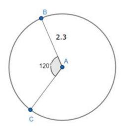
Step3: Using protractor draw a line perpendicular to AB from point B because tangent is perpendicular to the radius. Thus this line is tangent to circle at point B
