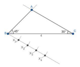
Step5: Join X<sub>3</sub> and C (3 being smaller of 4 and 3 in  $\frac{4}{3}$  and not X<sub>4</sub> because the ratio  $\frac{4}{3}$  is greater than 1)
