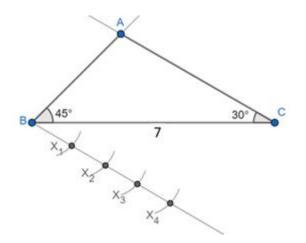
Step5: Join X<sub>3</sub> and C (3 being smaller of 4 and 3 in  $\frac{4}{3}$  and not X<sub>4</sub> because the ratio  $\frac{4}{3}$  is greater than 1)
