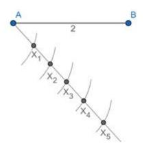
Step4: Join  $X_3B(X_3$  because the segment AB should be 3 parts). Extend AB and draw a line parallel to  $X_3B$  which intersects the extended AB at C. Hence C divides externally the segment AB
