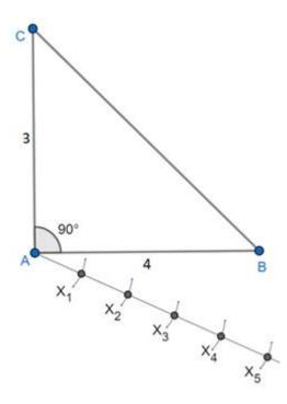
Step5: Join X<sub>3</sub> and B (3 being smaller of 5 and 3 in  $\frac{5}{3}$  and not X<sub>5</sub> because the ratio  $\frac{5}{3}$  is greater than 1)
