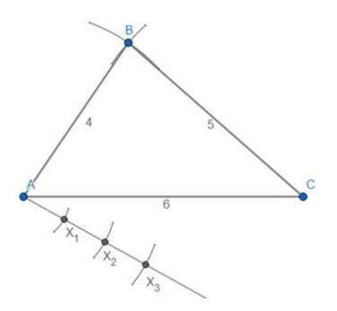
Step6: join  $X_3$  and C and from  $X_2$  (because  $X_2$  is the second point 2 being smaller in 2/3) construct line parallel to  $X_3C$  and mark the intersection point with AC as D
