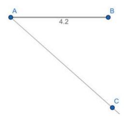
Step3: take any distance in compass and keep the needle of the compass on point A and draw an arc intersecting the line AC. Name the intersection point as  $X_1$ . Keeping the distance same in compass keep the needle on point  $X_1$  and mark an arc intersecting AC at  $X_2$ . Draw 8 (5:3 given ratio 5 + 3 = 8) such parts i.e. upto  $X_8$
