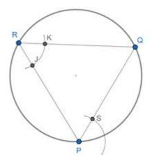
Step5: Measure the distance of arc JK in compass, keep the needle on point S and mark an arc intersecting the arc drawn in step4 at point T. Draw line passing through point P and T and it is the tangent.
