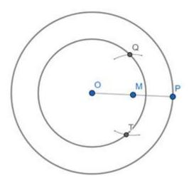
Step6: Construct a line passing through PQ and PT which are the required tangents and measure the lengths PQ and PT using a scale
