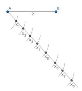
Step4: Join X<sub>5</sub>B. Extend AB and draw a line parallel to X<sub>5</sub>B which intersects the extended AB at C. Hence C divides externally the segment AB
