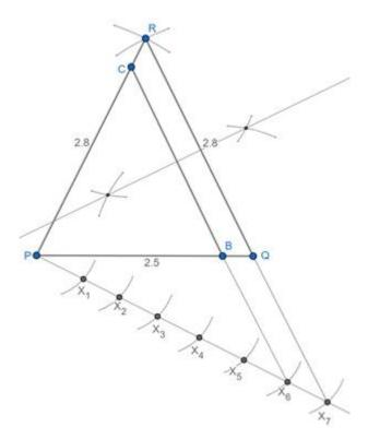
Step9: Repeat step7 and step8 to draw perpendicular bisector for PC and mark the intersection point of both perpendicular bisectors as O
