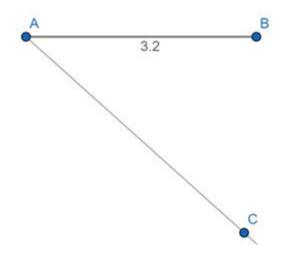
Step3: take any distance in compass and keep the needle of the compass on point A and draw an arc intersecting the line AC. Name the intersection point as  $X_1$ . Keeping the distance same in compass keep the needle on point  $X_1$  and mark an arc intersecting AC at  $X_2$ . Draw 8 (3:5 given ratio 3 + 5 = 8) such parts i.e. upto  $X_8$
