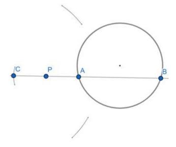
Step4: Keeping the distance in the compass same as that of in step3 keep the needle on B and mark arcs intersecting the arcs drawn in step3. Join these intersection points we get the perpendicular bisector of CB at M
