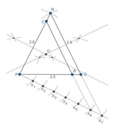
Step10: Keep the needle of the compass on point O and draw circle taking radius OC. Circumcentre of  $\Delta$ PBC is ready
