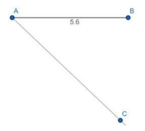
Step3: take any distance in compass and keep the needle of the compass on point A and draw an arc intersecting the line AC. Name the intersection point as  $X_1$ . Keeping the distance same in compass keep the needle on point  $X_1$  and mark an arc intersecting AC at  $X_2$ . Draw 13 (5:8 given ratio 5 + 8 = 13) such parts i.e. upto  $X_{13}$
