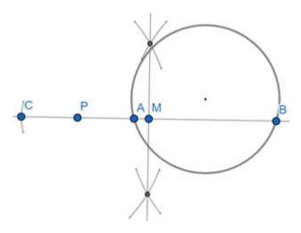
Step5: Take distance MB in compass keep the needle on point M and draw a semicircle as shown
