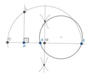
Step7: Take distance PL in compass, keep the needle on P and mark arc intersecting the circle at Q and T. Join PT and PQ thus PT and PQ are the required triangles
