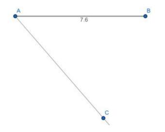
Step3: Take any distance in compass and keep the needle of the compass on point A and draw an arc intersecting the line AC. Name the intersection point as  $X_1$ . Keeping the distance same in compass keep the needle on point  $X_1$  and mark an arc intersecting AC at  $X_2$ . Draw 13 (5:8 given ratio 5 + 8 = 13) such parts i.e. upto  $X_{13}$
