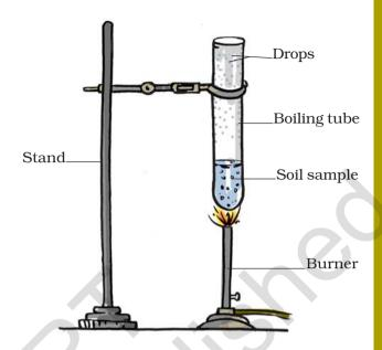
Fig. 9.6 Removing moisture from the soil
