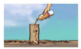
Fig. 9.5 Measuring rate of percolation
