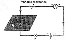
**Conclusion**: The direction of the north pole of the compass needle would give the direction of the field lines produced by the electric current through the straight wire at that point. **The direction of the field** is perpendicular to the plane of the coil and directed inwards for the clockwise current flowing. For anticlockwise current, it will be outwards.
