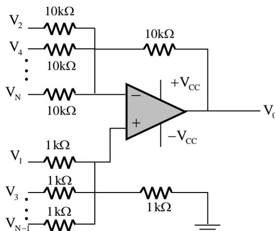
The voltages  $V_1, V_2, V_3, V_4, V_5, V_6, \dots$  are  $1, -1/2, 1/3, -1/4, 1/5, -1/6, \dots$  volt, respectively. As  $N$  approaches infinity, the output voltage (in volt) is \_\_\_\_\_.
