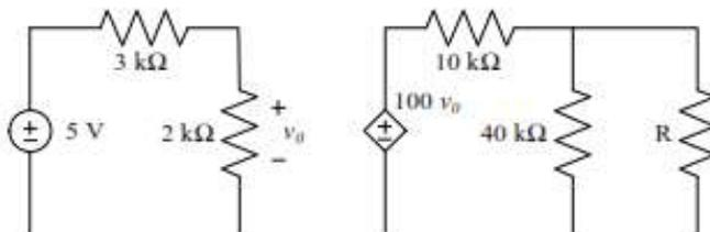
the maximum power (in watt) delivered to the resistor R is \_\_\_\_\_.
