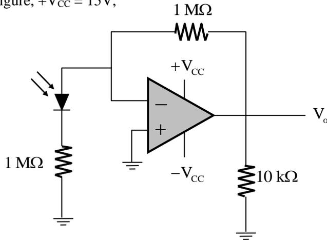
$-V_{CC} = -15\text{V}$ , Load resistor  $R_L = 10\text{k}\Omega$ . If  $10\mu\text{W}$  of power is incident on the photodiode, then the value of the photocurrent (in  $\mu\text{A}$ ) through the load is \_\_\_\_\_.
