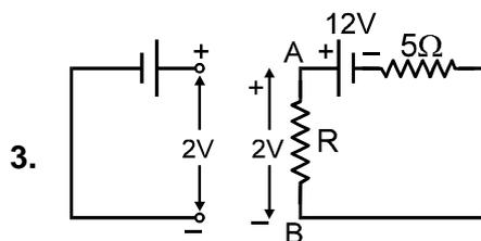
If pot. drop between A and B is also 2V, then no current will pass through the galvanometer.
