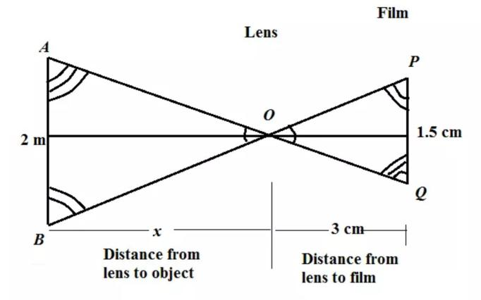
When we take a picture, the image of the object being photographed is projected by the camera lens on to the film. The height of the image on the film can be related to the height of the object using the similar triangle.
