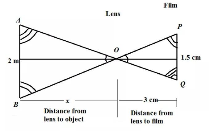
Since the corresponding angles of the given figure are in equal measure so, the triangles ABO and PQO are similar.
