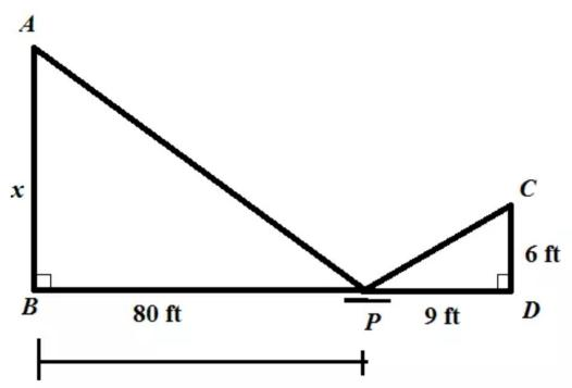
To solve the problem it can be assumed that the triangles ABP and CDP are similar triangle. By using the side proportionality condition, the height of the building can be estimated.
