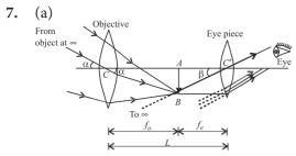
(b) For a telescope, lens  $L_1$  is chosen as objective, as its aperture and focal lengths are largest. The lens  $L_3$  is chosen as eyepiece as its focal length is smallest.
