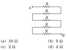
**40**. In the given circuit, the current in each resistor is
