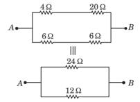
The equivalent resistance between A and B is
