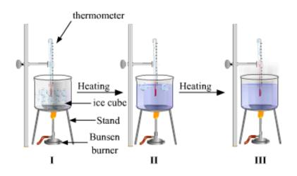
**Result**: In the beginning, the temperature of ice is below 0°C. When ice begins melting, the temperature is recorded to be 0°C. Temperature remains constant at 0°C till all the ice melts. The continued heating of water causes its temperature to rise.
