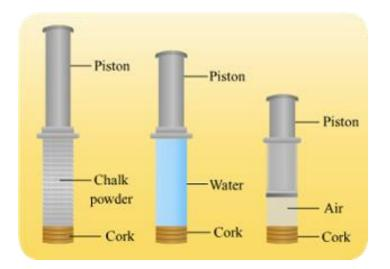
**Result:** The force required to push the pistons of syringes containing chalk powder and water will be greater than that required to push the piston of the syringe containing air.
