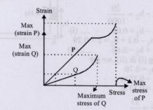
The strain of P is more than Q therefore P is more ductile.
