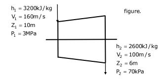
51. If mass flow rate of steam through the turbine is 20kg/s, the power output of the turbine (in MW) is
