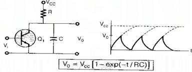
where,  $V_0$  = Instantaneous voltage across the capacitor at time t; V  $V_{cc}$  = Supply voltage
