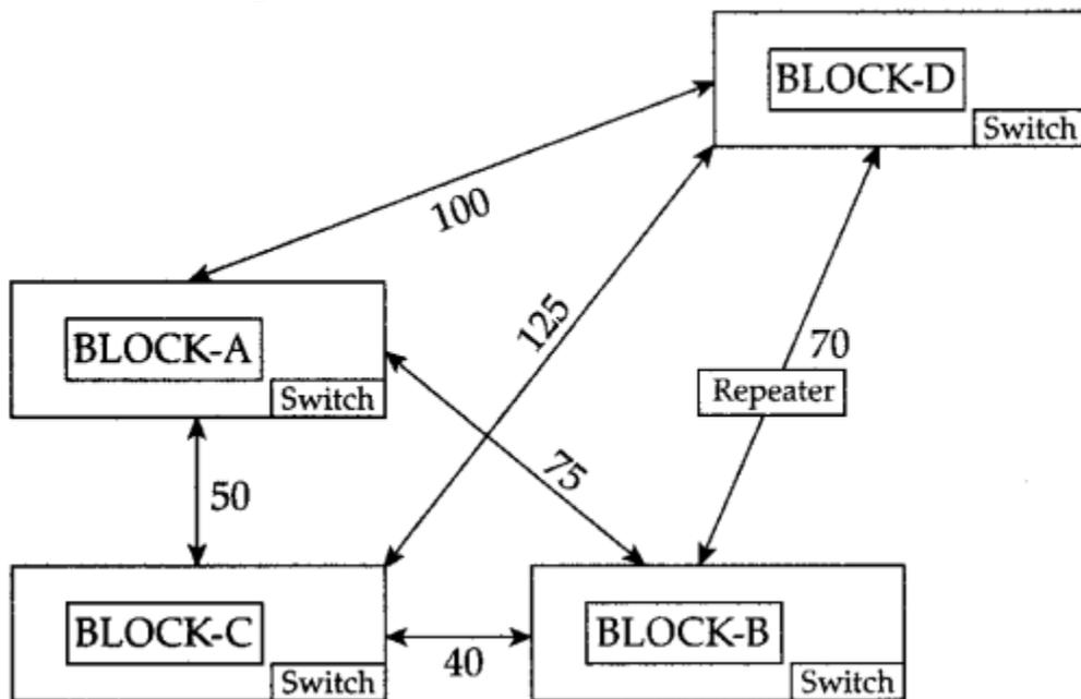
3. Switch is a device used to segment network into different sub-networks so switch will exist in all the blocks. Since distance between BLOCK-D and BLOCK-C is large so repeater will be install between BLOCK-D and BLOCK-C.
