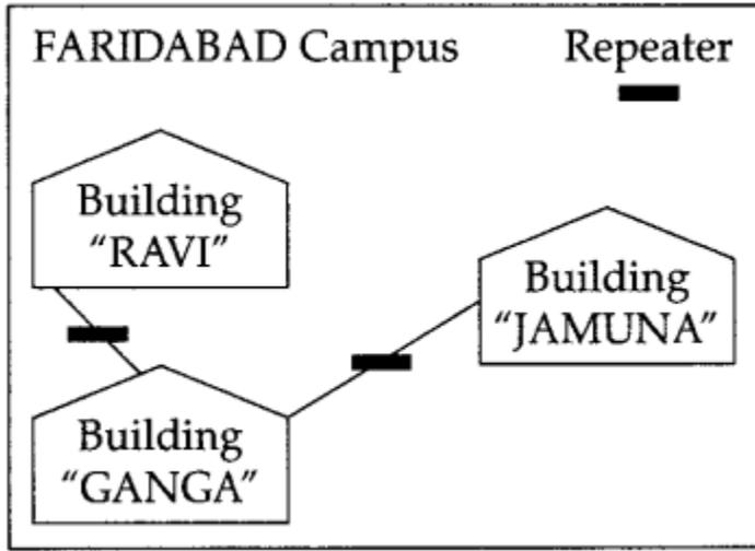
3. (a) Since the cabling distance between buildings GANGA and JAMUNA are quite large, so a repeater each, would ideally be needed along their path to avoid loss of signals during the course of data flow in these routes.
