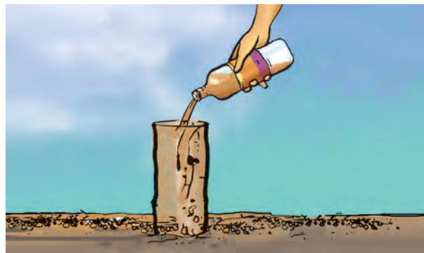
Fig. 9.5 Measuring rate of percolation
