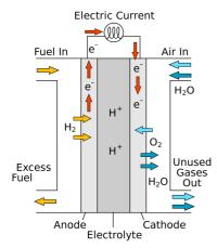
The electrode reactions involved in the working of the H<sub>2</sub>-O<sub>2</sub> fuel cell are as:
