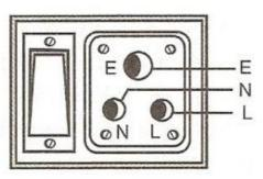
E: for earth pin N: for neutral wire pin L: for live wire pin.
