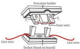
The figure above shows the most common fuse arrangement in which the fuse wire is stretched between the two metallic terminals  $T_1$  and  $T_2$  in a porcelain holder. This holder fits into a porcelain socket having two metallic terminals to each of which the live wire of the circuit is connected.
