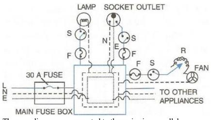
These appliances are connected to the mains in a parallel arrangement.
