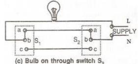
Similarly if the bulb is in on position as shown in Fig. (b) or (c), one can switch off the bulb either from the switch  $S_1$  or the switch  $S_2$ .
