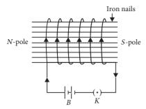
(b) The magnetism of soft iron inside the solenoid disappears immediately after switch off the current while steel does not and it becomes a permanent magnet. Therefore, core of electromagnet must be of soft iron but not steel.
