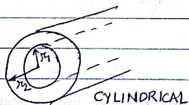
$$\frac{2\pi KL(T_1 - T_2)}{\ln\left(\frac{r_2}{r_1}\right)}$$
