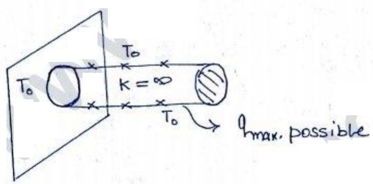
$$\left. \begin{matrix} T_{entire} \\ \text{Surface} \end{matrix} = T_0 \right\}$$
