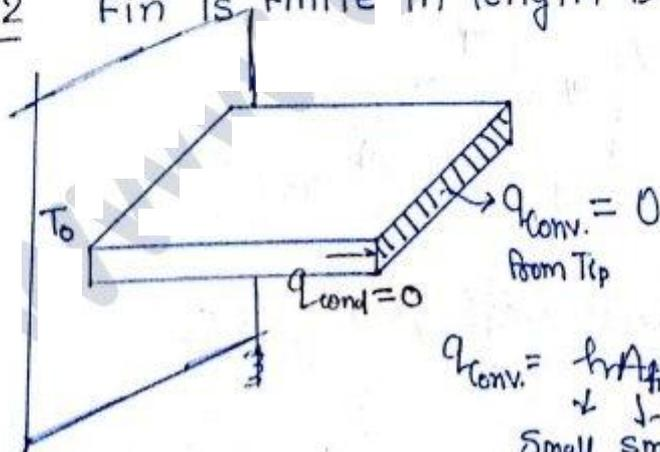
Heat conduction into the tip of fin = 0
