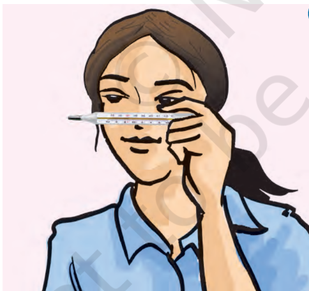
Fig. 4.3 Correct method of reading a clinical thermometer
