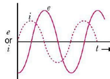
78. The phase difference between the alternating current and emf is  $\frac{\pi}{2}$ . Which of the following can not be the constituent of the circuits?
