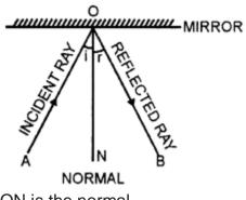
ON is the normal ∠AON is the angle of incidence ∠NOB is the angle of reflection.
