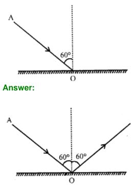
Law of reflection of light is used to draw the direction of the reflected ray. This law states that angle of incidence is equal to the angle of reflection.  $\angle i = \angle r$
