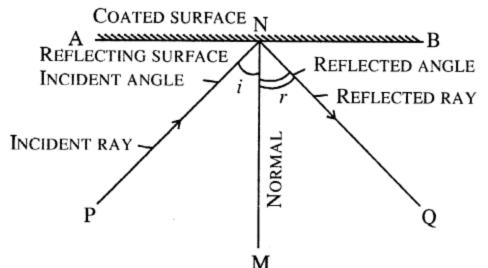
Angle of incidence— The angle formed between the incident ray and the normal is the angle of incidence. (PNM is the angle of incidence.)
