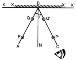
Fix two steel pins P and Q on the straight line AB atleast 10 cm apart. Look for the images of the pins P and Q and fix two pins P Q' such that P', Q' and images of P and Q are all in the same straight line. Remove the pins and draw small circles around the pin pricks.
