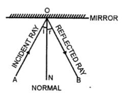
ON is the normal ∠AON is the angle of incidence ∠NOB is the angle of reflection.
