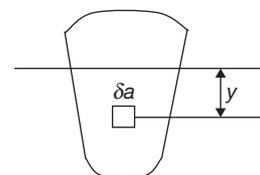
$$q = \frac{dM}{dx} \frac{1}{bI} \int_y^{y'} da, \text{ where } da = bdy = \text{area of the element.}$$
