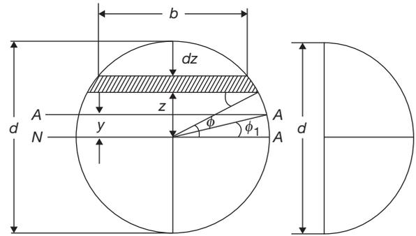
In the given circular section of diameter  $d$ , shear stress is to be determined at a section  $AA$  at a distance  $y$  from the neutral axis  $NA$ . For finding the moment of the area above  $AA$ , an element of thickness  $dz$  at a vertical distance  $z$  from neutral axis is considered.
