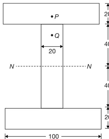
The shear stress at point  $P$  (very close to the bottom of the flange) is 12 MPa. The stress at point  $Q$  in the web (very close to the flange) is
