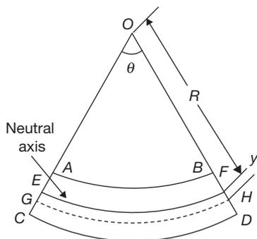
After bending, cross-sections  $AC$  and  $BD$  subtend an angle  $\theta$  at  $O$ . Let,  $R$  be the radius of the neutral plane represented by  $EF$ . Then,  $EF = R\theta$ .
