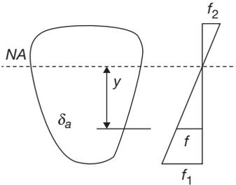
Stress is varying linearly across the depth. Consider an element area  $\delta a$  at a distance  $y$  from the neutral axis. Let  $f$  be the stress on this area.
