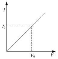
Straight line graph between potential difference(V) and current(I) shows that resistor is a linear element and follows Ohm's Law.
