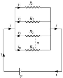
Let there are *n* resistances, each of value  $R_1, R_2, \dots, R_n$ , respectively, are connected in parallel to a battery of voltage *V*. if the equivalent resistance of the circuit is  $R_{eq}$ , then current drawn from the battery is  $i = \frac{V}{R_{eq}}$ . The total current *i* then divides into  $i_1, i_2, i_3, \dots, i_n$ , respectively in the given resistors.
