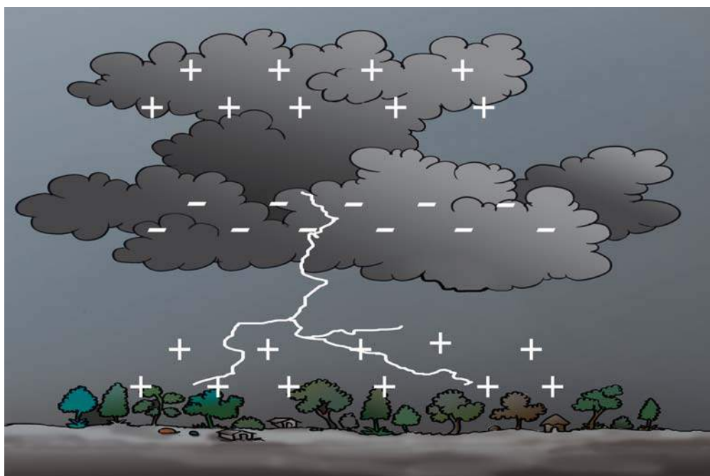
Fig 15.5 : Accumulation of charges leading to lightning.
