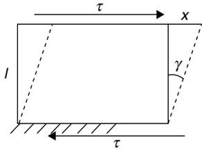
Shear stress causes an angular deformation. The change in the right angle of the element is known as shear strain. It is denoted by the angle  $\gamma$ . From the figure,
