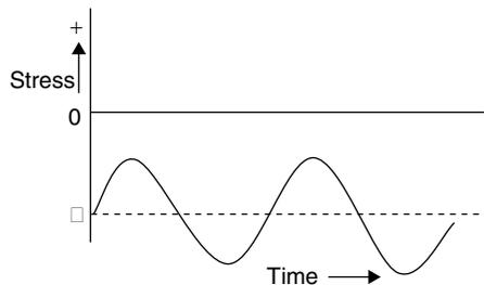
Type (3) is the general case of fluctuating stress. When the amplitude is equal in positive and negative sides as in the case (4), it is called a completely reversed stress.
