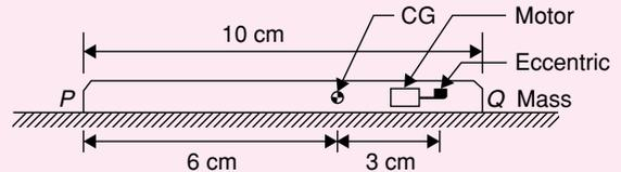
Given in addition that the eccentric mass = 2 grams, eccentricity = 2.19 mm, mass of mobile = 90 grams,  $g = 9.81 \text{ m/s}^2$ . Uniform speed of the motor in RPM for which the mobile will get just lifted off the ground at the end Q is approximately [2015]
