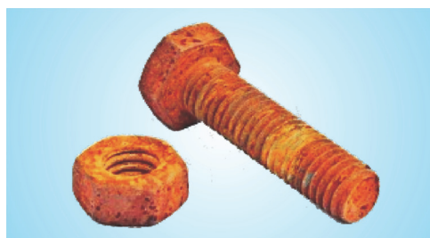
Fig. 4.9: Rusty nuts and bolts of iron
