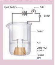
of a 6V battery through a bulb and a switch as shown in Figure. Now pour some dilute HCl in the beaker and switch on the current. Repeat the activity with dilute sulphuric acid, glucose and alcohol solutions. What do you observe now? Does the bulb glow in all cases?
