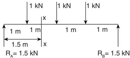
Shear force at the section  $xx$  is  $1.5 - 1.0 = 0.5 \text{ kN}$
