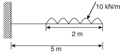
The displacement of the free end of the cantilever beam shown in figure is
