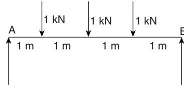
A simply supported beam *AB* is loaded as shown in the figure. The beam has a rectangular cross section of 100 mm width and 240 mm depth.
