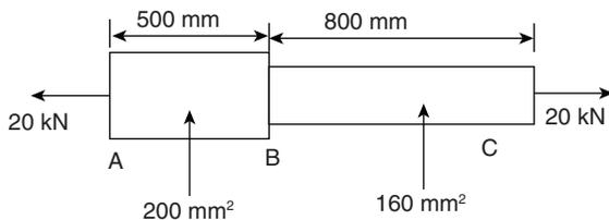
A bar  $ABC$  with cross sectional area  $200 \text{ mm}^2$  at portion  $AB$  and  $150 \text{ mm}^2$  at portion  $BC$  is subjected to an axial pull of 20 kN. If  $E = 2 \times 10^5 \text{ N/mm}^2$ , strain energy stored in the bar is
