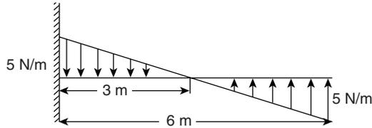
A cantilever beam of 6 m span is subjected to a uniformly varying load as shown. The bending moment at the middle of the beam is
