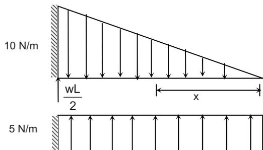
Bending moment due to uniformly varying load at  $x = 3$  m.
