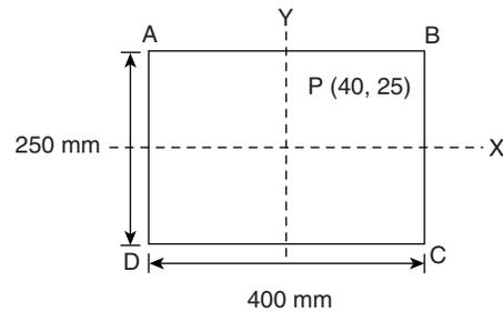
On a short masonry column of cross section as shown above, a concentrated load of 500 kN is applied at point P, + 40 mm from y axis and + 25 mm from x – axis. Moment of inertia about x– axis = 520.833 × 10<sup>6</sup> and moment of inertia about y – axis = 1333 × 10<sup>6</sup>
