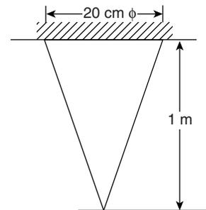
If specific weight is  $80000 \text{ N/m}^3$  and modulus of elasticity is  $E = 2 \times 10^5 \text{ N/mm}^2$ , extension of its length due to self weight is
