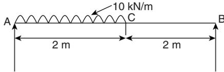
The simply supported beam loaded as shown above has a flexural rigidity 833.33 kN – m<sup>2</sup>
