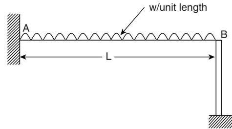
The free end of the cantilever  $AB$  is supported by a prop. The cantilever is loaded by a uniformly distributed load as shown in the figure. Assuming that there is no deflection at the free end, force on the prop is
