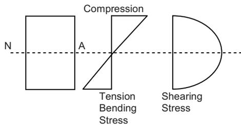
Shearing stress is maximum at neutral axis
