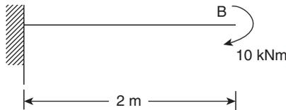
A cantilever AB of length 2 m and 100 mm breadth and 200 mm depth is fixed at end A. It is subjected to a moment of 10 kNm at the free end B. Flexural rigidity is 13,340 kN–m<sup>2</sup>. Magnitude of maximum deflection is
