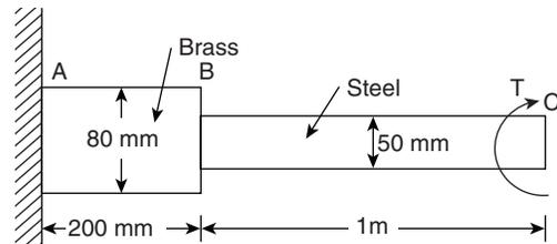
For the stepped shaft *ABC*, fixed at *A*, portion *AB* is made of brass and portion *BC* is made of steel, Allowable shear stress for brass is 80 N/mm<sup>2</sup> and for steel is 100 N/mm<sup>2</sup>. Modulus of rigidity for brass is 40 kN/mm<sup>2</sup> and for steel is 80 kN/mm<sup>2</sup>
