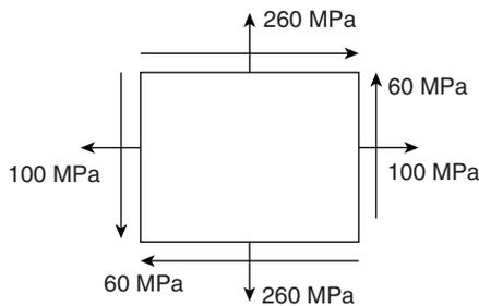
Figure shows state of stress at a point in a stressed body. Radius of Mohr's circle representing the state of stress is
