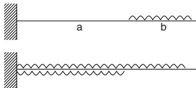
The given uniformly distributed loading of the cantilever can be treated as a combination as shown above. i.e., a full loading + a negative loading through length  $a$
