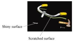
Try to scratch the shiny coating of the handle of a bicycle. You will find that the surface beneath is dull. **Do you know how the handle bar of a bicycle is made so shiny?**
