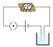
You can test whether liquids allow current to pass through them or not by observing the deflection of a magnetic compass needle.
