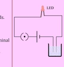
Air is a bad conductor of electricity. Thus, we do not get a shock standing at a distance from a wire carrying current. Minerals naturally present in water make it a good conductor of electricity since salt solutions can conduct electricity. Hence, it is advisable not to touch an electrical appliance with wet hands.
