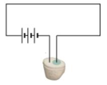
Since potato is a good conductor of electricity, it allows the current to pass through it. Hence, the current flows through the circuit. Leave the circuit for about 25 minutes. Observe the inserted place of the potato carefully. **Do you notice a greenish-blue spot on the potato around the positive electrode?**
