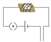
A magnetic compass needle experiences a force and deflects when a current carrying a wire is placed near it.
