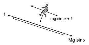
For plank be at rest, applying Newtons second law to plank along the incline
