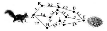
The Shortest way to reach the grains is the AGFKE path.
