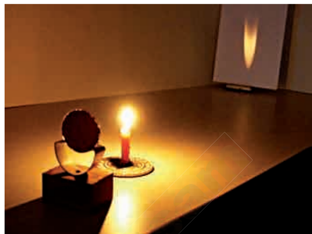
Fig. 15.15 Real images formed by a concave mirror
