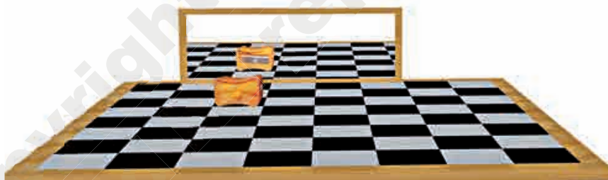
Fig. 15.7 Locating image in a plane mirror
