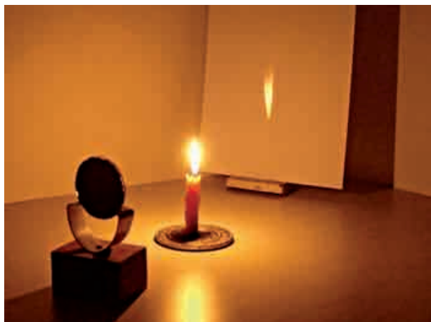
Fig. 15.15 Real images formed by a concave mirror
