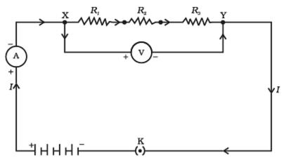
(i) What does the diagram show regarding the arrangement of resistors?Ans: The diagram shows that the resistors are connected end-to-end in a single path, one after the other, forming a series circuit.
