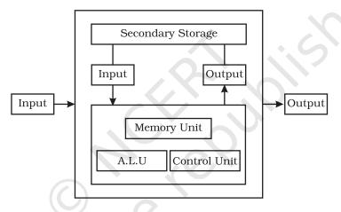
Fig. 12.1 : Block diagram of main components of computer
