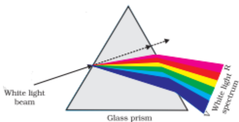
Figure 11.5 Dispersion of white light by the glass prism
