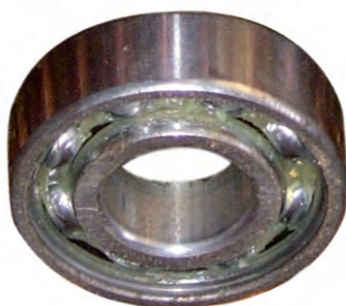
Fig. 12.16 : Ball bearings reduce friction
