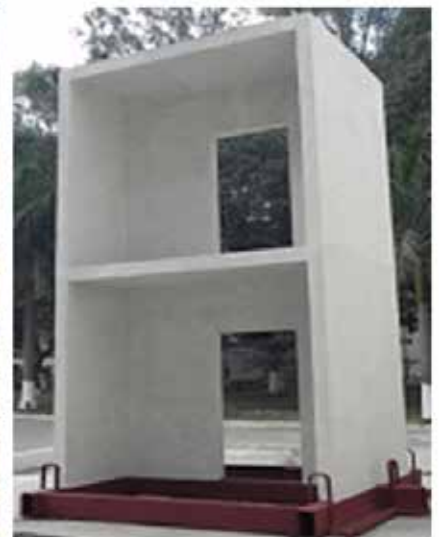
Spraying and pouring of concrete over the EPS core skeleton and finished building model
