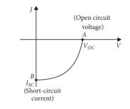
(i) *V-I* curve is drawn in the fourth quadrant, because a solar cell does not draws current but supply current to the load.
