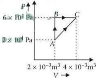
In process AB, 400 J of heat is added to the system and in process BC, 100 J of heat is added to the system. The heat absorbed by the system in the process AC will be
