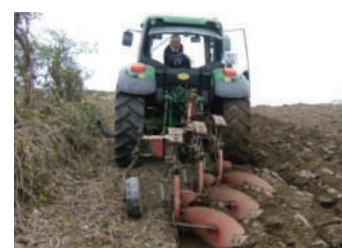
Deep chisel plough works up to 20 cm depth Source: www.tootoo.com
